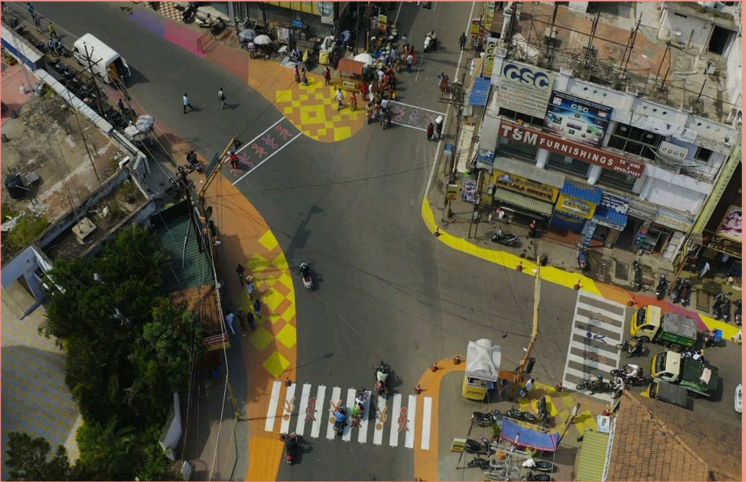
Figure 15: Transformation of Big Bazaar Street that improves edge management and promotes safe crossings 20
